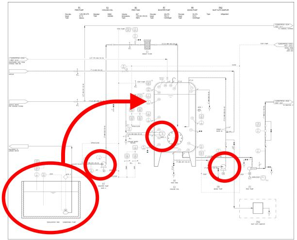
The feeding tank is insulated and equipped with a coil cooling system and a steam heating system.
