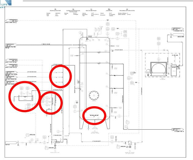
Nitrogen recirculation takes place thanks to K1 blower and 9 microbubble plates placed at the base of the reactor, capable of distributing the nitrogen uniformly and keeping the granules under stirring
